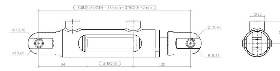
NOTE: ALL THREADS MACHINED TO 2A/B SPECIFICATION. ALL PIN HOLES MACHINED TO D9 TOLERANCE.
